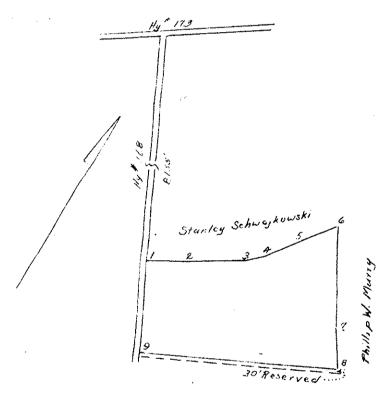
Beginning at a point (1), said point being on Highway No. 168 8155' distance from the intersection of Highways No. 168 and 173.
