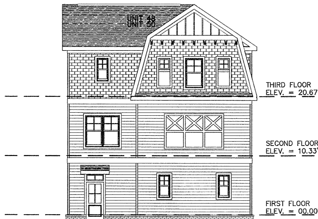
REAR ELEVATION (PUBLIC STREET SIDE)
